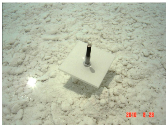
Fig. 3. Photograph at one of the experimental sites. The sample holder represents the Wucaichi pool site location with still water conditions.
