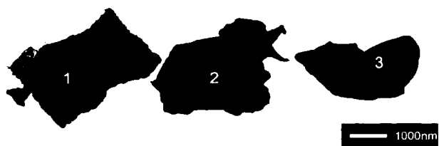
Figure 4 — TEM photograph of minerals in Guizhou Bayer red mud. 1: quartz, 2: halite, 3: almandite.
