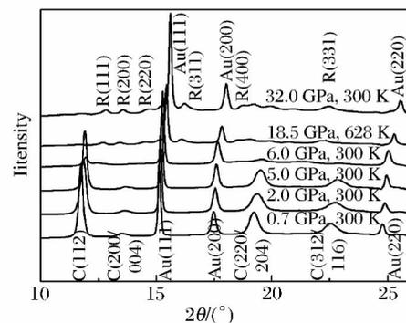
C; Chalcopyrite structure peak; R; Rocksalt structure peak
