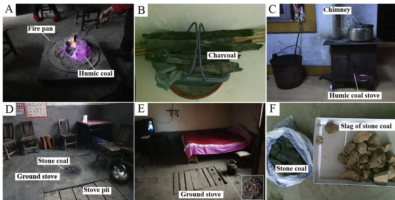
Fig. 2. On-site sampling of different types of solid fuels. (A), fire pan at family #8; (B), charcoal sample at family #4; (C), iron stove for humic coal at family #2; (D), ground stove at family #8; (E), ground stove at family #9; (F), stone coal and its slag.
