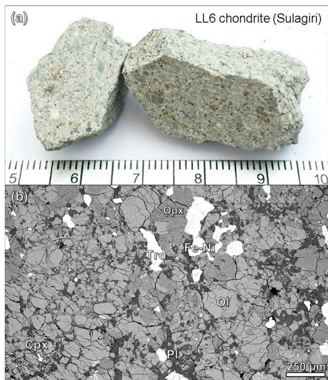
Fig. 2. (a) Hand sample of LL6 chondrite meteorite Sulagira, weighing ~17 g; (b) BSE image of the representative area of Sulagiri, showing this meteorite is mainly composed of olivine (Ol), orthopyroxene (Opx), clinopyroxene (Cpx), plagioclase (Pl), troilite (Tro), and Fe-Ni metal (Fe-Ni).
