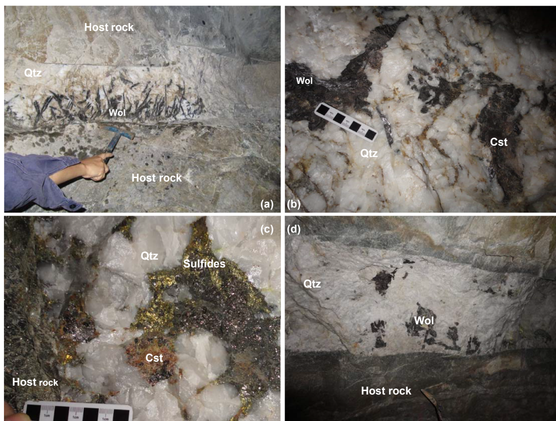
Fig. 3. Photographs of ore and gangue minerals in vein system. Wol: wolframite, Qtz: quartz, Cst: cassiterite.
