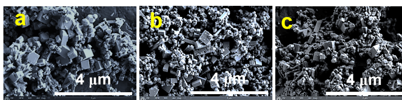
Figure 7. SEM images of the as-synthesized pyrite crystals at 24 h with Na 2 S and S powder as the sulfur source: (a) 5 mmol/L Na 2 S + 5 mmol/L S powder, (b) 10 mmol/L Na 2 S + 10 mmol/L S powder, and (c) 15 mmol/L Na 2 S + 15 mmol/L S powder.
