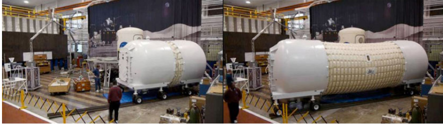
Fig. 20.20 Deployment Testing of the X-Hab Lunar Habitat at NASA LaRC (credit: NASA / ILC Dover)
