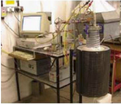
Fig. 7.5 Laboratory rig used in the Ilmenox project, showing electric furnace with tubular metal retort and electrochemical equipment.
