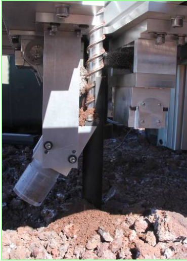
Fig. 10.10 Sampling system allows bringing up of regolith samples directly to a cup or analysis instrument.
