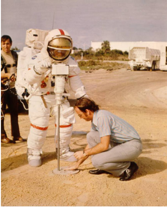
Fig. 10.6 Apollo astronaut practices drilling using the Apollo Lunar Surface Drill. Image courtesy: NASA
