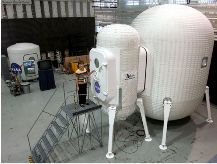
Fig. 20.15 The planetary surface habitat and airlock unit (credit: NASA / ILC Dover)
