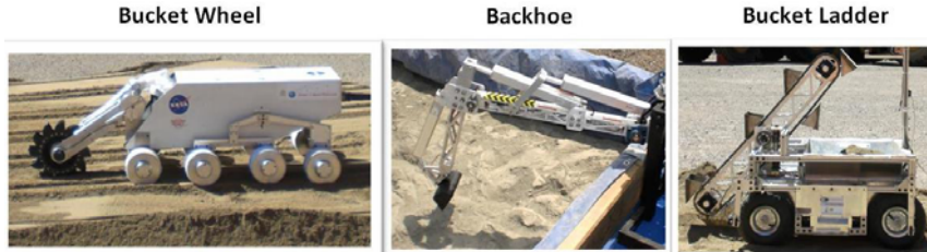
Fig. 10.8 Example of various types of excavators developed at the Colorado School of Mines. Photo courtesy Paul van Susante.
