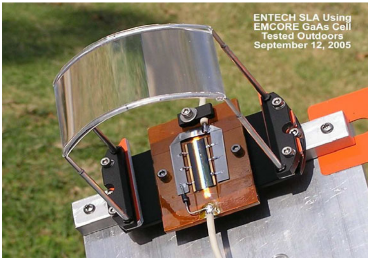
Fig. 25.16 SLA Module with GaAs Cells
