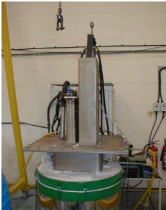
Fig. 7.6 Pilot plant rig used in the Ilmenox project, showing electric furnace with rectangular metal retort supporting the anode chamber (left) and cathode chamber (right).
