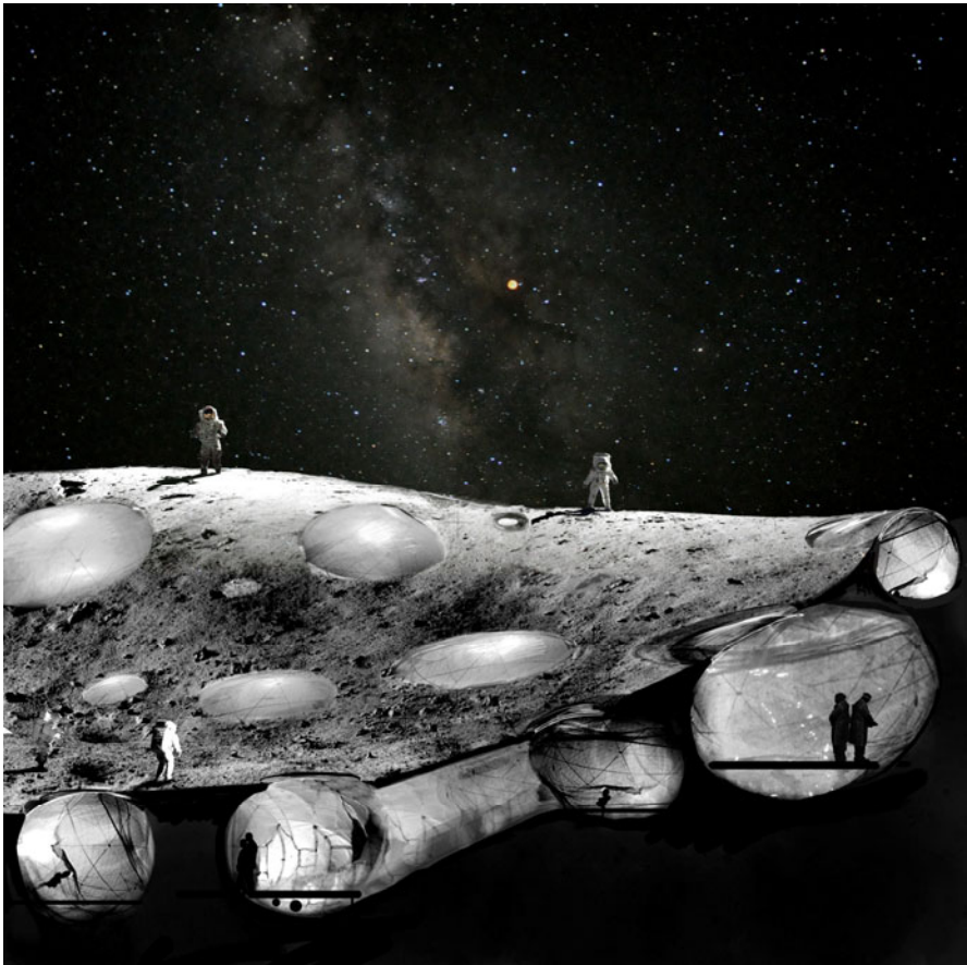
Fig. 28.7 The entire inflatable insertion can be used as an initial mould for the regolith structure to wrap around
