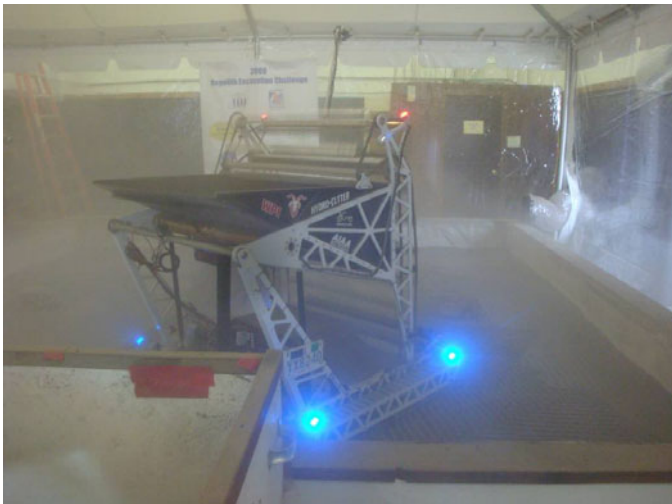
Fig. 10.13 Paul's Robotics lunar excavator ready for its first dump. During the 30 minute period, teleoperated excavator, called the Moonraker, collected and dumped 439 of regolith. The four blue LEDs were installed a few days before the competition to aid in navigation. Photo courtesy K. Zacny.
