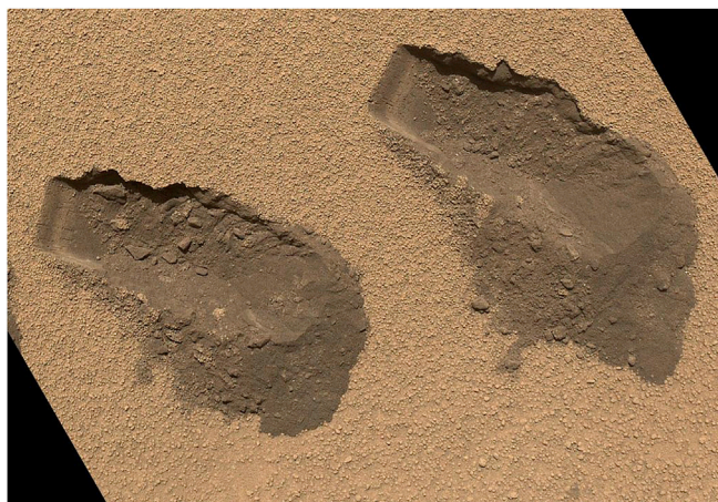
Fig. 5. View of the third (left) and fourth (right) trenches made by the 4-cm-wide scoop on NASA's Mars rover Curiosity in October 2012. The image was acquired by the Mars Hand Lens Imager (MAHLI) on Sol 84 (Oct. 31, 2012) and shows some of the details regarding the properties of the "Rocknest" wind drift sand (Credit: NASA/JPL-Caltech/MSSS. URL http://mars.jpl.nasa.gov/msl/multimedia/images/?ImageID=4917 ).
