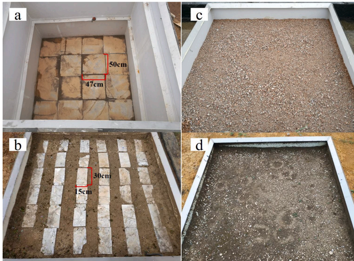
Fig. 3. Interior filling diagram of different rock-soil structures.
