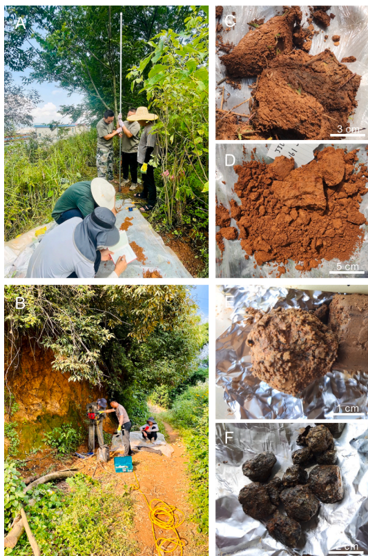
Fig. 4. Field photos of the drilling techniques and core samples of different parts of regolith profile. (A) Sampling by the soil auger. (B) Sampling by the backpack rotary drill. (C) Top humic layer samples. (D) Typical pedolith samples. (E) Saprolite samples. (F) Saprock samples.
