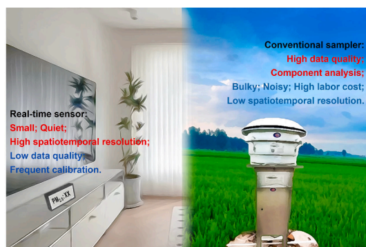
Fig. 1. The comparison of indoor real-time monitor and conventional sampler.
