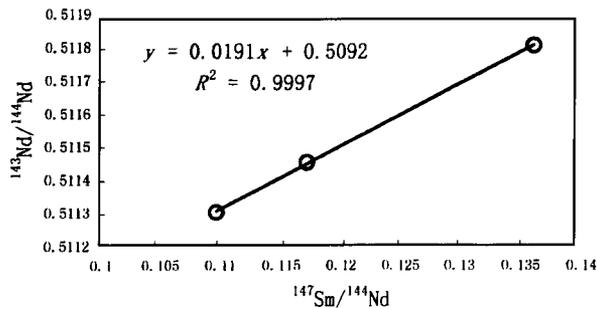
Fig. 3. Whole-rock Sm-Nd isochron diagram of the Se'ertengshan greenstone.
