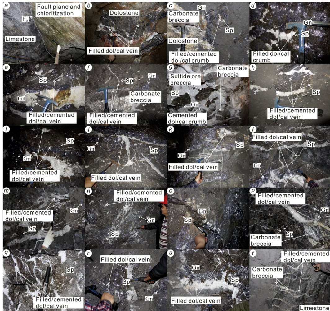
Fig. 4. Field photographs of the Fule deposit; a: F_6 reverse fault plane with chloritization; b: post-ore dolomite/calcite (Dol/Cal) veins fill fractures in dolostone; c: sphalerite (Sp) and galena (Gn) occur as massive aggregates that are filled by Dol/Cal crumbs, and carbonate breccias are cemented by Dol/Cal veins; d: Dol/Cal occur as crumbs and fill fractures in massive Sp and Gn aggregates; e: massive Sp and Gn aggregates are filled/cemented by Dol/Cal veins; f: massive Sp and Gn, and carbonate breccias are filled/cemented by Dol/Cal veins; g: breccias of sulfide ore and carbonate are cemented by Dol/Cal crumb aggregates; h: interbedded sulfide veins are filled/cemented by Dol/Cal veins or veinlets; h–n: massive Sp and Gn are filled/cemented by Dol/Cal veins; o: massive Sp and Gn; p: Dol/Cal veins fill fractures in the wall rocks or cement carbonate breccias, and Sp and Gn occur as speckles or single crystals that are irregularly distributed in the wall rocks; q–r: massive Sp and/or Gn are filled/cemented by Dol/Cal veins; t: post-ore Dol/Cal veins fill fractures in the wall rocks or cement the carbonate breccias.
