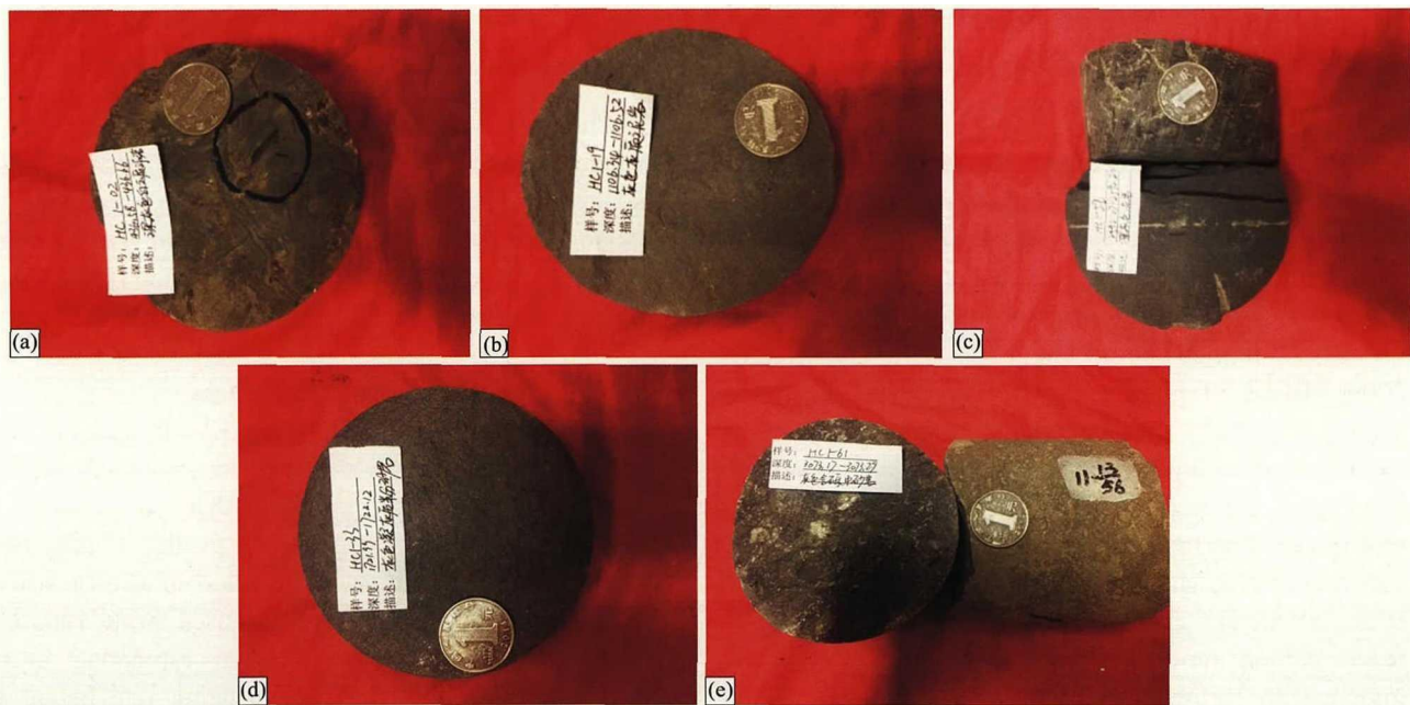
Fig. 2. Photos of cores taken from the Hari sag. (a), Depth: 436 m, stratum: K 1y , lithology: mudstone; (b), Depth: 1106m, stratum: K 1s , lithology: mudstone; (c), Depth: 2592m, stratum: K 1b , lithology: mudstone; (d), Depth: 1722m, stratum: K 1s , lithology: gray sandstone; (e), Depth: 3073m, stratum: K 1b , lithology: gray sandstone.
