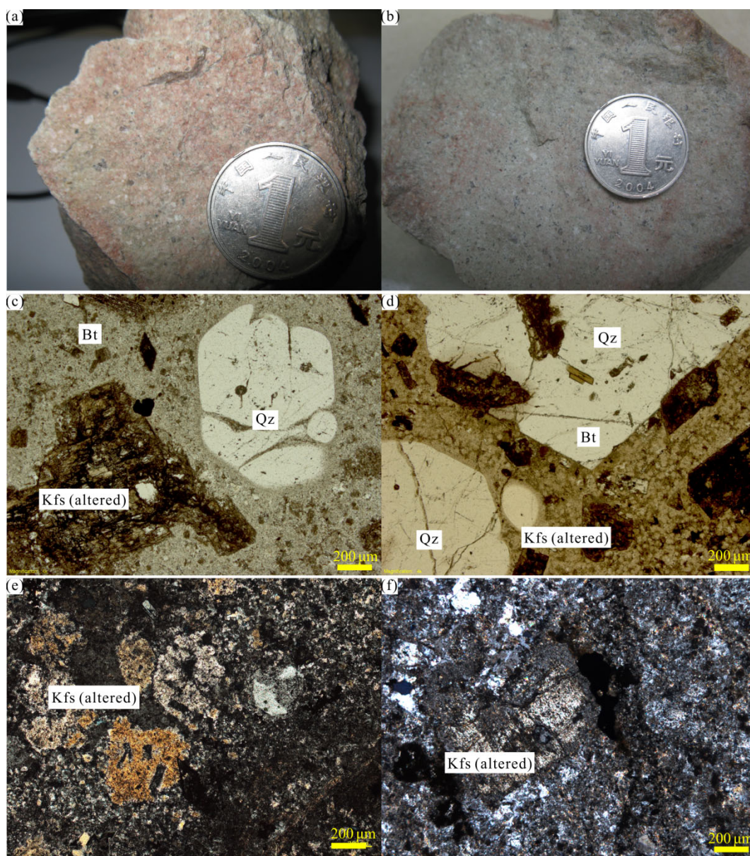
Figure 4. Hand specimen and microscope photos of the Houyaoyu granite porphyries. (a), (b) are hand specimen showing that they are massive structure and porphyritic texture; (c), (d) are photomicrograph showing that the Houyaoyu granite porphyries with classic porphyritic texture consist of quartz (Qz), K-feldspar (Kfs), biotite (Bt), apatite, sphene, pyrite (Py), magnetite. Furthermore, phenocrysts consist of quartz, K-feldspar and biotite, and the same is true for matrix composition; (e), (f) are photomicrograph from YY-22 and YY-56.
