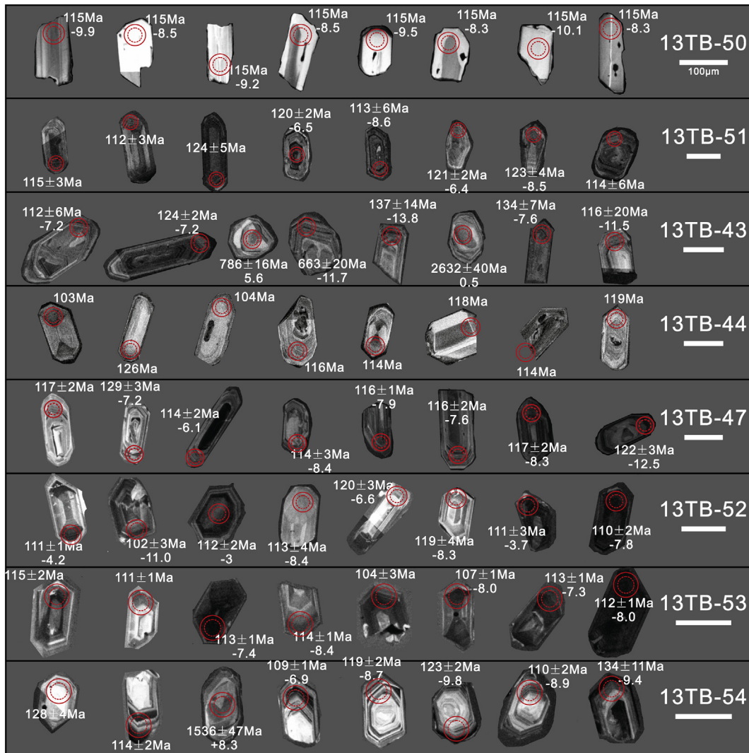
Fig. 6. Cathodoluminescence images of the representative zircons from the Lushui-Pianma Batholith. Scale bar = 100 μm; small circles are of laser U–Pb analysis and large circles of Hf isotope analysis; the numbers nearby represent U–Pb ages and \epsilon_{\text{Hf}}(t) values, respectively.
